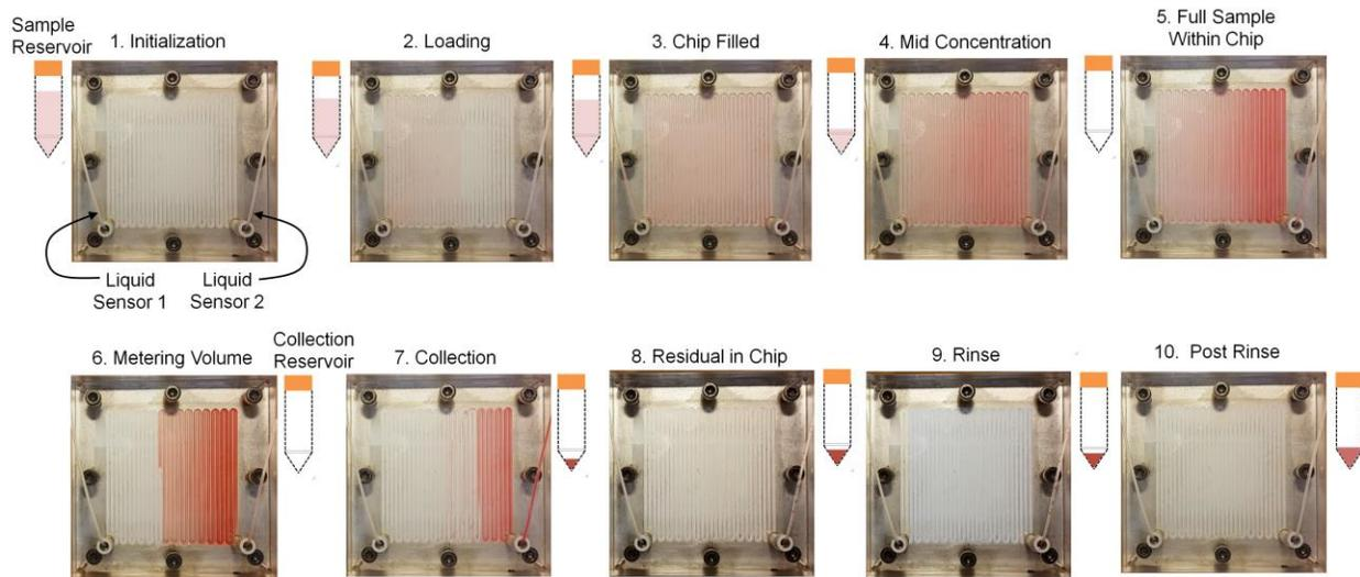
**Figure 2-3: Photographs showing system operation during the concentration process for a sample of diluted food dye**
