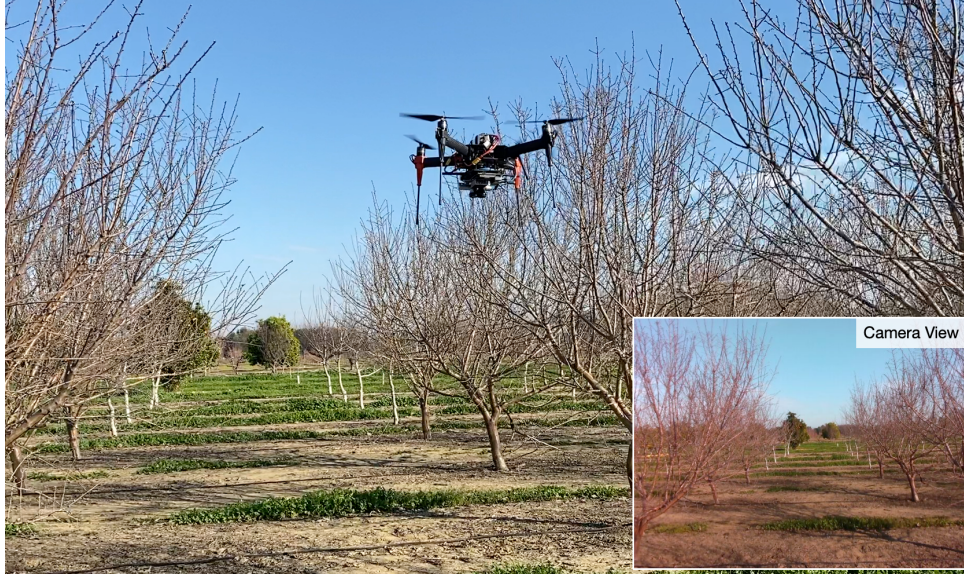
Figure 5.1: The drone is flying autonomously in this orchard without GPS and knows how to avoid the tree branches along the way. The view of onboard camera is provided.
