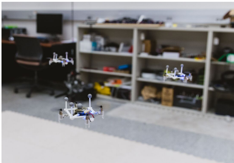
Figure 1.2: Example of multirotor UAVs taking off and landing in ground effect regions.
