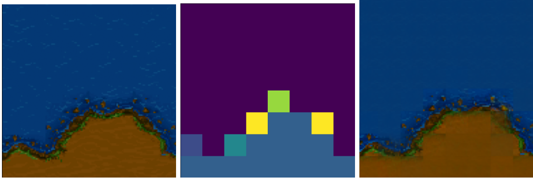
Figure 11.4: The autoencoder model reconstructs colored images after passing them through a bottleneck of discrete latent codes. Left, original data from WarCraft II map. Middle, the discrete latent variables in the bottleneck layer of the VQ-VAE. Right, the reconstructed image from the latent variables.
