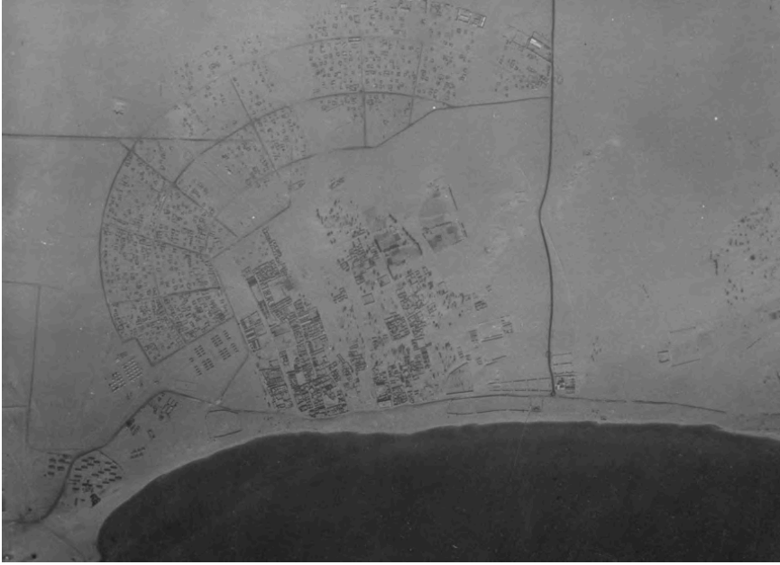
Figure 2.14 This aerial photograph of Ahmadi from 1954 clearly shows the juxtaposition of the development of Badawiyah to the south of the original KOC enclave to the north, which is characterized by semi-circular avenues bisected by radial roads and uniformly laid out housing plots. South Ahmadi is characterized by a road grid, but built structures are arranged organically and without evidence of the formal pattern of settlement in the enclave.
