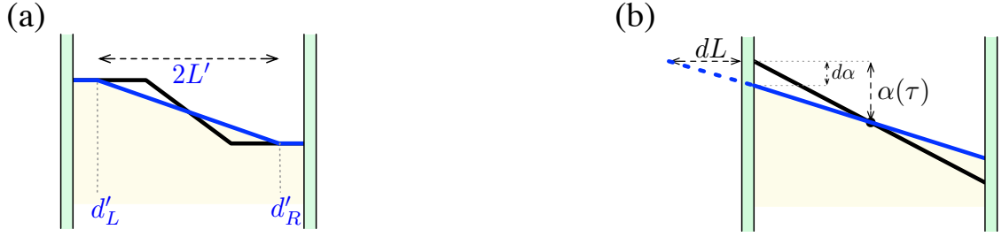
Figure 2.5: Updating the concentration profile in a straight channel in (a) case 1, and (b) case 2. The “before” profile is black and the “after” profile is blue.
