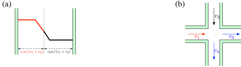
Figure 2.8: (a) Splitting an SP-function into two SP-functions (red and black). (b) A join-and-split node.
