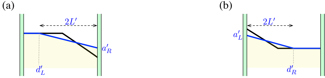
Figure 2.6: Updating the concentration profile in a straight channel in (a) case 3, and (b) case 4.
