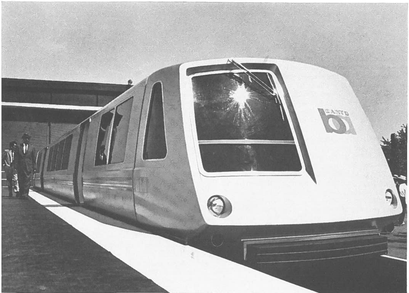
FULL-SCALE MODEL of a BARTD train was photographed at the test station near Concord, Calif. The detachable forward pod has space for an attendant and automatic-control equipment. The at-
