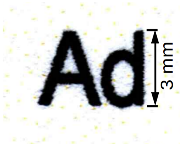
Figure 7.1: A magnified view of two printed letters surrounded by yellow dots. These two letters happen to be located inside one of the rectangles used for FPM-DPPM.
