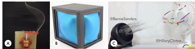
Figure 1: a) LightWire, an illuminated, spinning optic fiber that forms light bodies from social data, b) GorgeBox, an object that inflates based on the accumulation of data, c) LiveFans, two IoT controllable objects that actuate relational data.
