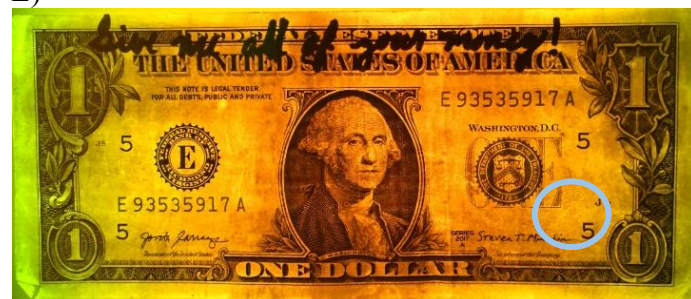
Figure 16: The best fingerprint quality for money samples. Fingerprint enhancement first with ninhydrin and then DNA analysis (mean quality of 3.4) (A). Fingerprint enhancement first with 1,2-indanedione and then DNA analysis (mean quality of 2.8) (B). DNA analysis first then fingerprinting with ninhydrin (mean quality of 2) (C-D). DNA analysis first then fingerprinting with 1,2-indanedione (mean quality of 2.8) (E).
