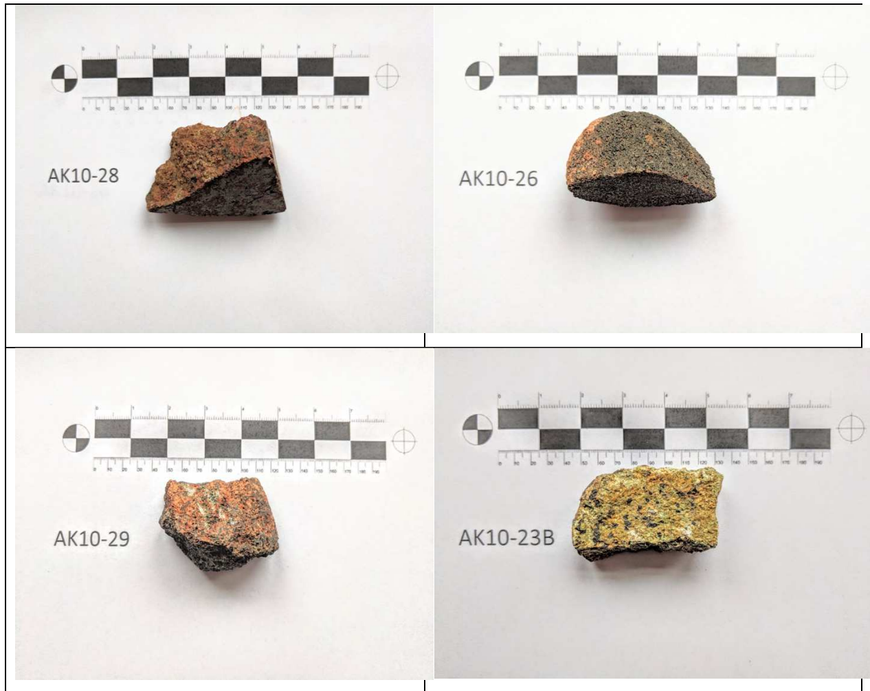
Figure 3: Hand specimens showing evidence of melt infiltration. Lithologies are as follows: olivine websterite (AK-1028), high-Al pyroxenite (AK-1026), pyroxenite (AK-1029), and lherzolite (AK-1023-B).
