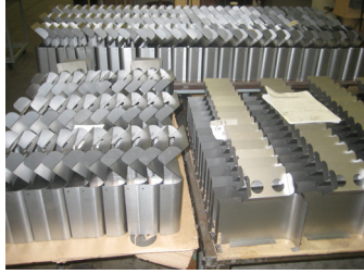
Laser-cut foot warmer pieces in the factory.
