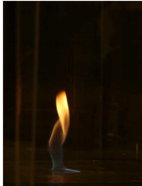
Figure 36: Both fins are at 10 degrees. It is very apparent the 2.00" pool is almost a blue whirl. The right illustration shows no vortex breakdown and is still a typical fire whirl.
