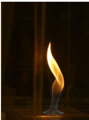
Figure 30: A helical fire whirl with fins at 20 degrees.
