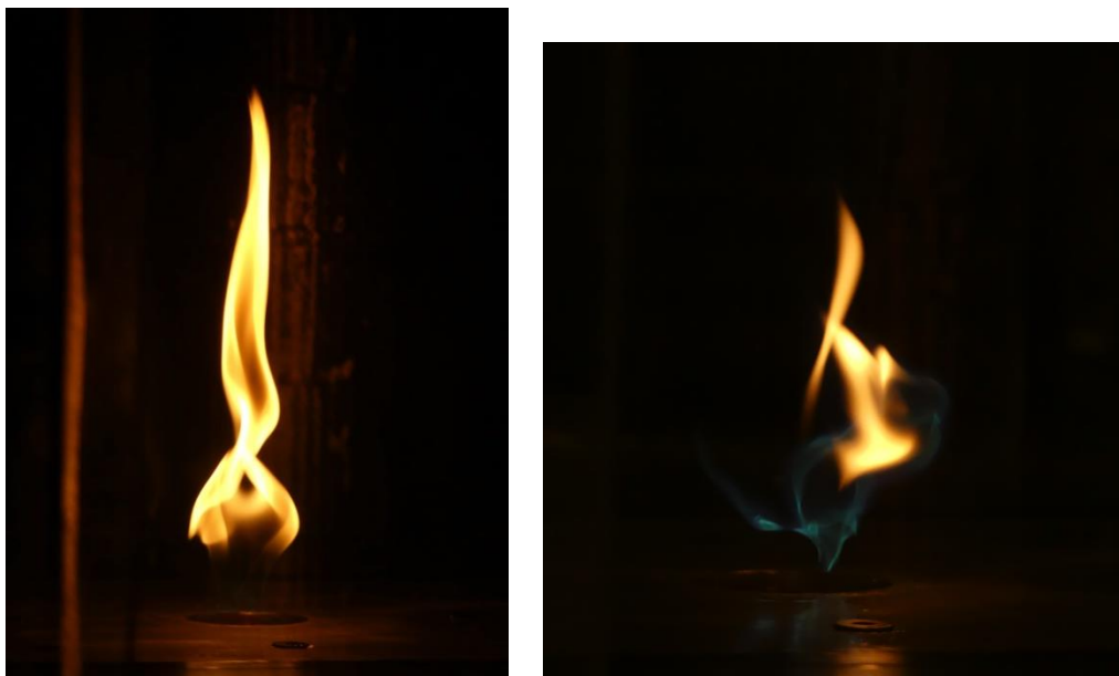
Figure 27: With the fins at 10 degrees, the vortex continued to break down while transitioning into a blue whirl.
