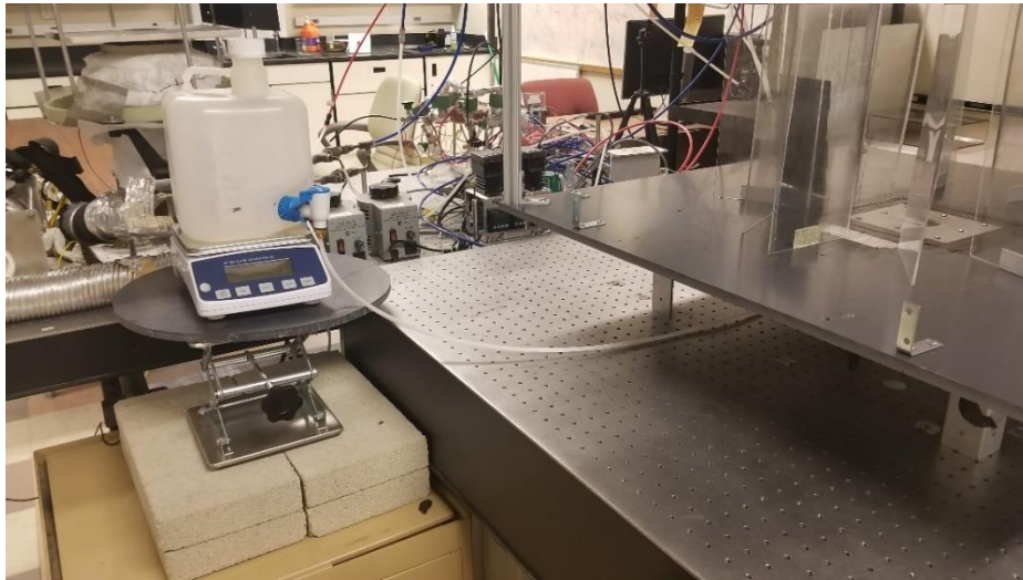
Figure 16: Scale and fuel container used for the experiment.
