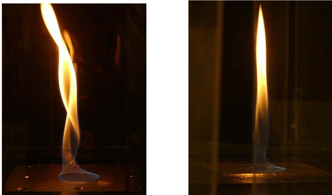
Figure 33: Both fins are at 40 degrees. The left is a 2.00" diameter pool and the right is a 1.25" diameter pool.
