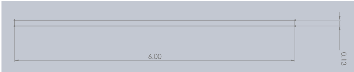
Figure 44: Side View of fin, dimensions are in inches
