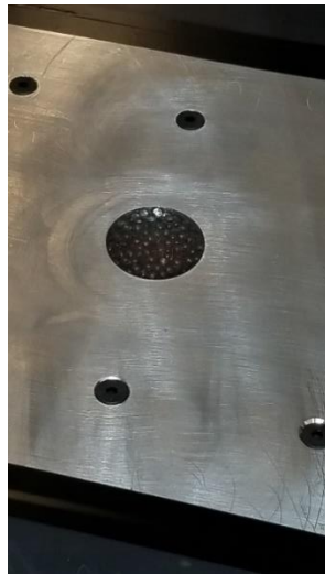
Figure 17: Glass beads placed within fuel reservoir.
