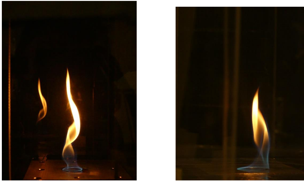
Figure 35: Fins at 20 degrees, 2.00" pool on left and 1.25" on the right. The shapes are very similar with the whirl on the left being more elongated.
