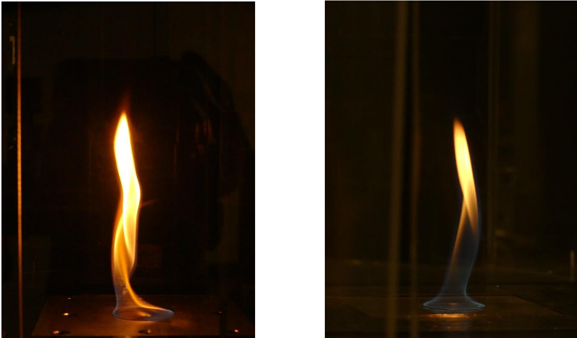
Figure 34: Fins at 30 degrees. The left is a pool size of 2.00" and the right is a pool size of 1.25", both using ethanol as a fuel source.
