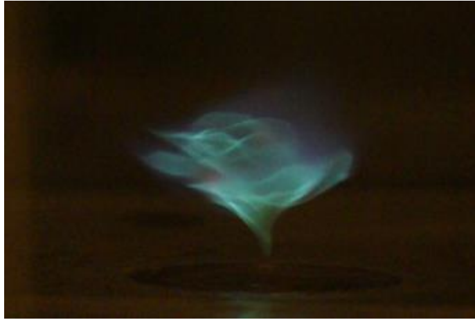
Figure 28: Blue whirl, 1.25" diameter with heptane fuel and fins at 5 degrees.
