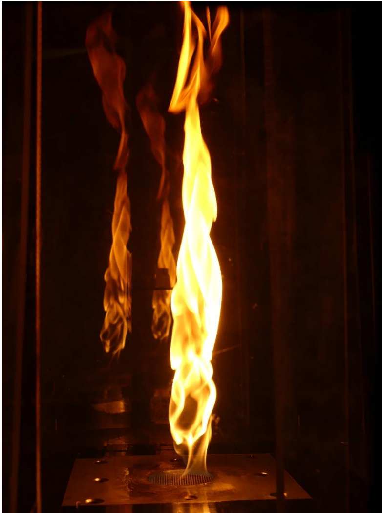
Figure 40: Yellow whirl with fins at 20 degrees and pool siz of 2.00"
