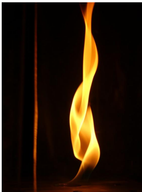
Figure 24: At 30 degrees, a very stable fire whirl is produced.
