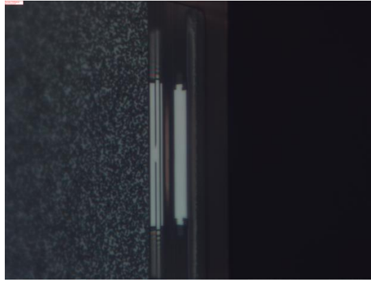
Figure 1.3.1. Zoomed section of the read-write portion on the ABS. Left part of the metal stripes are reader shields, and the writer return poles are on the right.
