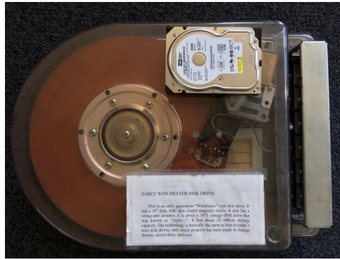
Figure 1.1.1 An early Winchester drive around 1975. It works on 14" disks and holds a storage capacity of 20 Mega-bytes. The "brown-orange" material on the disk is the hue of iron oxide particles. Its size is considerably huge compared to a more modern Western Digital 3.5" drive manufactured in 2008 with 40 Giga-bytes capacity on the top-right of the figure.
