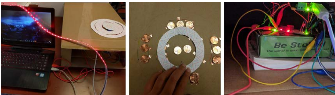
Figure 3. 18 Cardboard prototype with coins and Makey Makey
