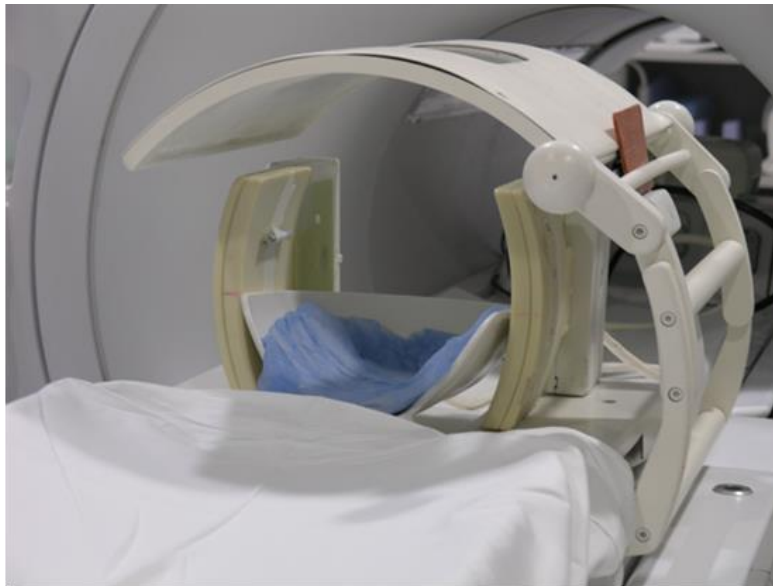
Figure 6.1 The coil setup of brain imaging study consists of a clamshell transmit and an 8-channel phased array receiver. (Figure from brain imaging manual.)
