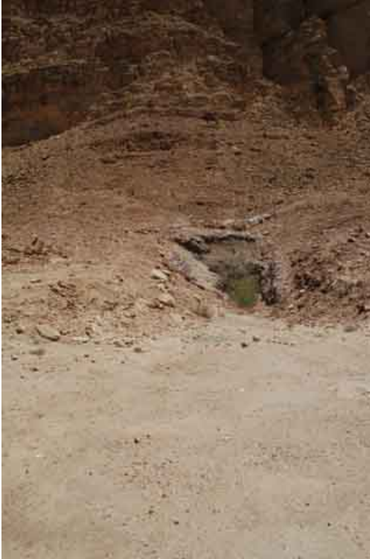
Figure 3.72: A mine opening at site 578. The opening has been enlarged by a bulldozer. The modern digging stops after about ten meters, after which the mine may open into a gallery or a shaft.
