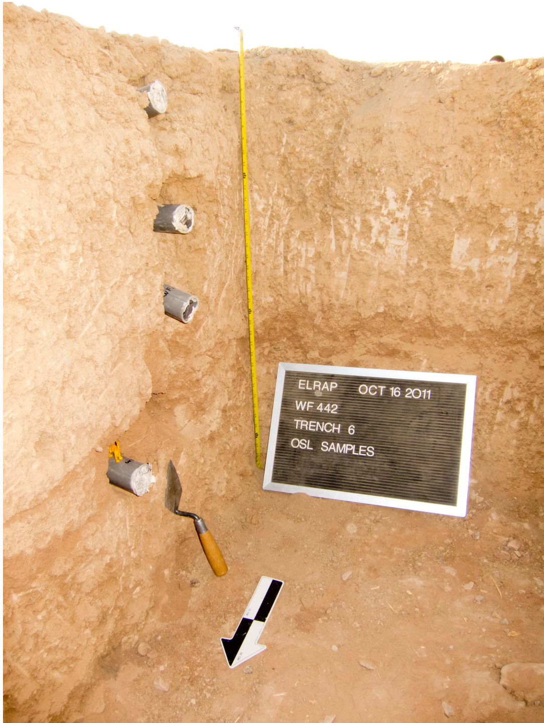
Figure 4.8: Image demonstrating the collection of OSL samples. Because they are light sensitive, the samples were collected before direct sunlight was hitting the profile, using PVC pipe hammered into the sidewall. The ends were packed with paper and wrapped in tinfoil and duct tape to prevent sediments from shifting and eliminate exposure to light.
