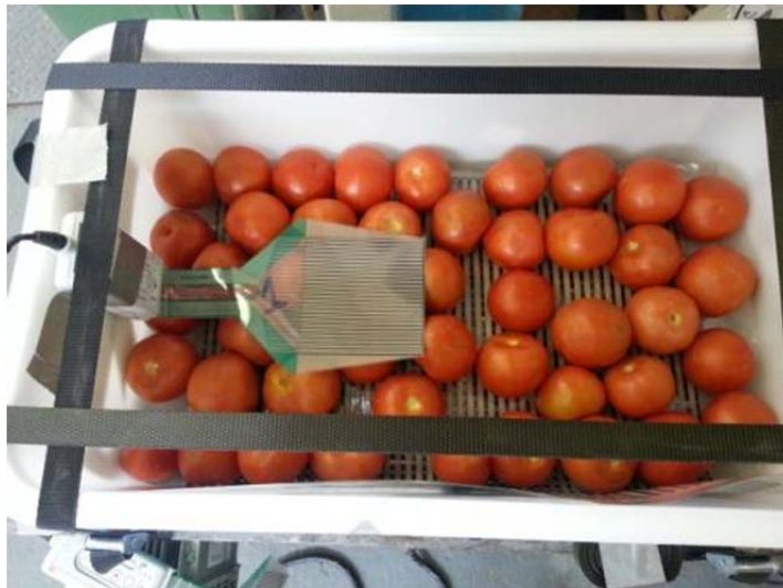
Figure 5.6: Bottom layer of tomatoes showing bottom and first layer pressure sensors in place.
