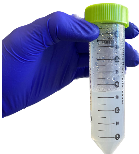
Figure 2: An example of the dextran, agarose gel phantom
