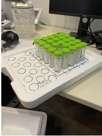
Figure 3: Custom foam phantom holder
