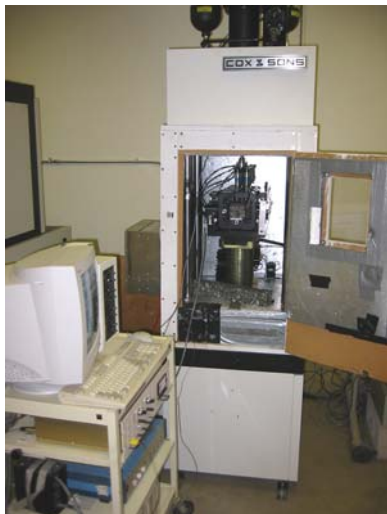
Figure 5: Moisture conditioning and flexural fatigue test equipment.
