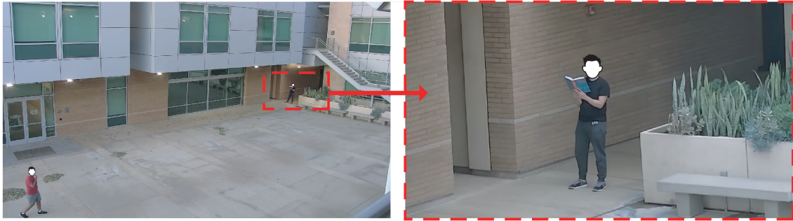
Figure 3.1: Zoomed out (left) and zoomed-in (right) views. The zoomed out view enables the detection of new targets as they enter the scene. However, it is insufficient for inferring target activities. The zoomed in view facilitates inferring target activities (i.e., a target reads a book) but only partially covers the scene. AcTrak balances zooming in and out such that target activities are captured, while ensuring that arriving targets are detected quickly when they step in to the scene.
