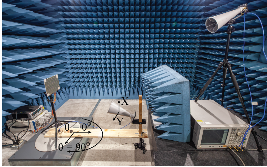
Figure 5.7. Experiment setup. \theta denotes the rotation angle of the Tx. X and Y indicate the direction of XP and YP.
