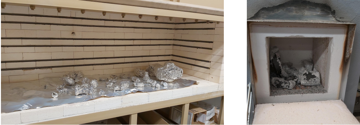
Figure 2.10: Left: parts after a successful hydrogen bake at the chemistry glassblowing shop. Right: parts destroyed in another hydrogen bake attempt.
