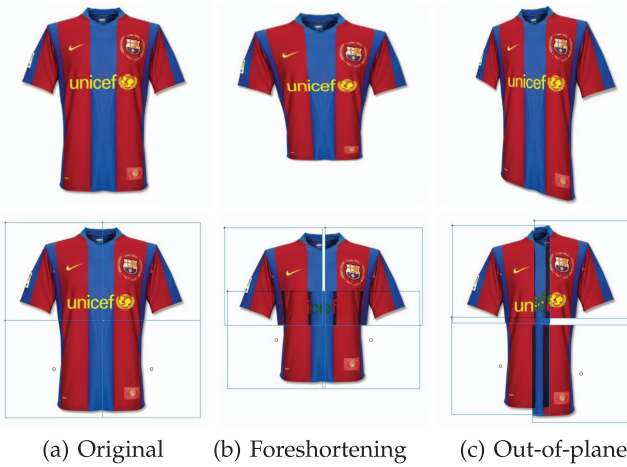
Fig. 2. We show that four small, translating parts can approximate nonaffine (e.g., perspective) warps.
