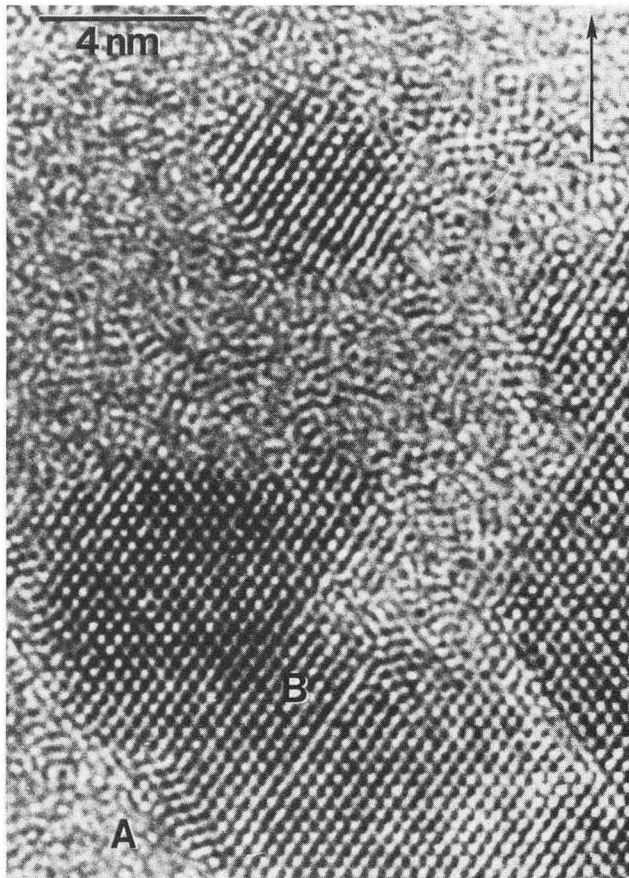
Figure 1-3. Cross-sectional HREM image ( \langle 110 \rangle orientation) of the amorphous-crystalline transition region in as-implanted GaAs (450-keV Se + into (100) GaAs, 1 \times 10^{14}/\text{cm}^2 dose, room temperature). (XBB 830-9399)
