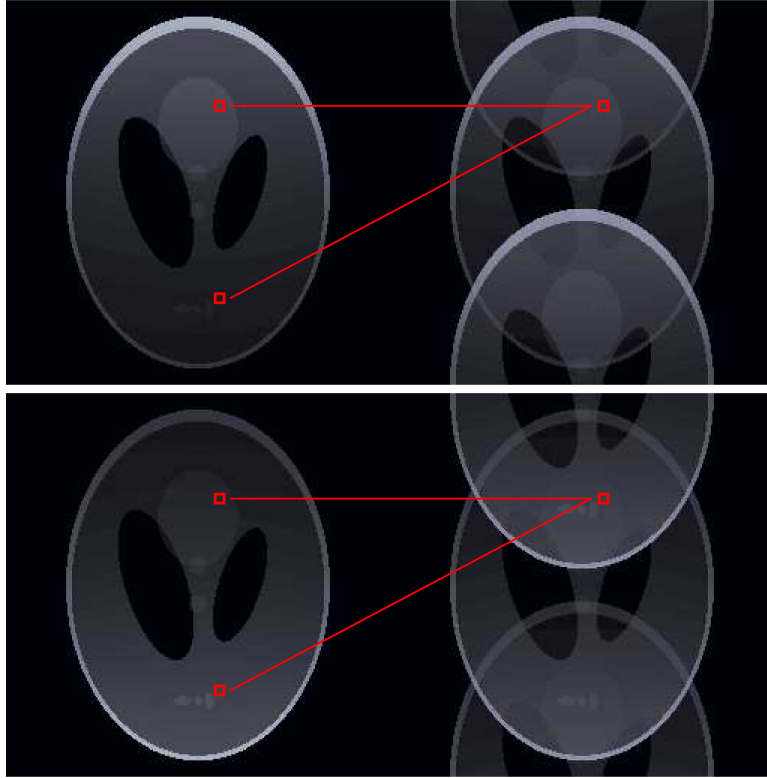
Figure 2.7: Sensitivity weighted images from a coil above the image (top) and one below the image (bottom). In the top image, the top pixel contributes more to the aliased pixel, while in the bottom image, it is the bottom pixel that contributes more.
