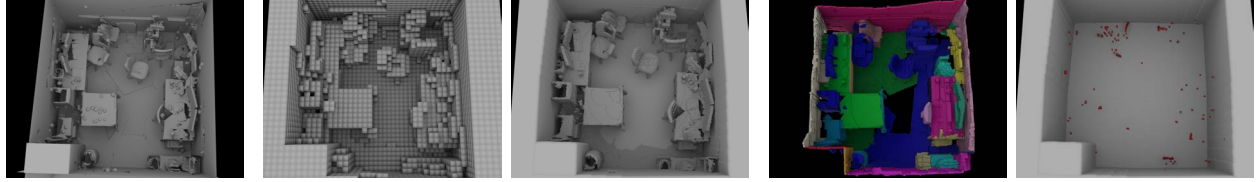
(a) input 3D scene (b) voxelized scene (low/high resolution) (c) segmentation (d) scanline-fill diff
