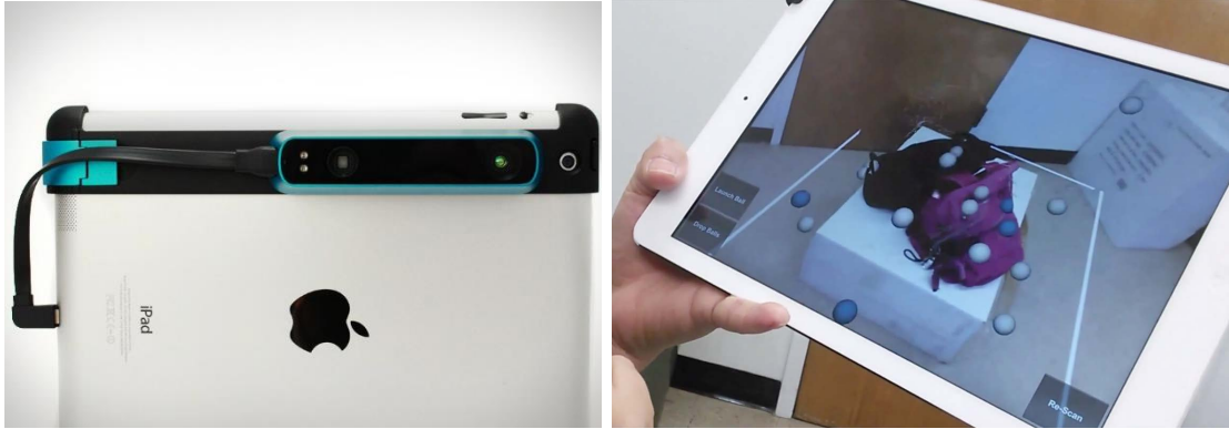
Figure 9.2: A 3D Structure Sensor attached to a tablet (left) and a physical simulation interface (right) are used in this work. The interface simulates a few balls falling onto a bag into a container.
