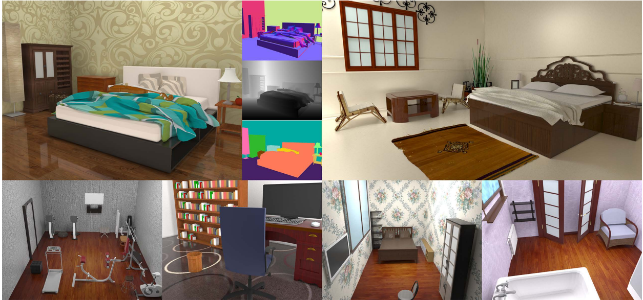
Figure 6.1: (Top Left) An example automatically-generated 3D bedroom scene, rendered as a photorealistic RGB image, along with per-pixel ground truth of surface normal, depth, and object identity. (Top Right) Another synthesized bedroom scene. Synthesized scenes include fine details—objects ( e.g. , the duvet and pillows on beds) and their textures are changeable, by sampling physical parameters of materials (reflectance, roughness, glossiness, etc. ), and illumination parameters are sampled from continuous spaces of possible positions, intensities, and colors. (Bottom) Rendered images of 4 example synthetic indoor scenes.
