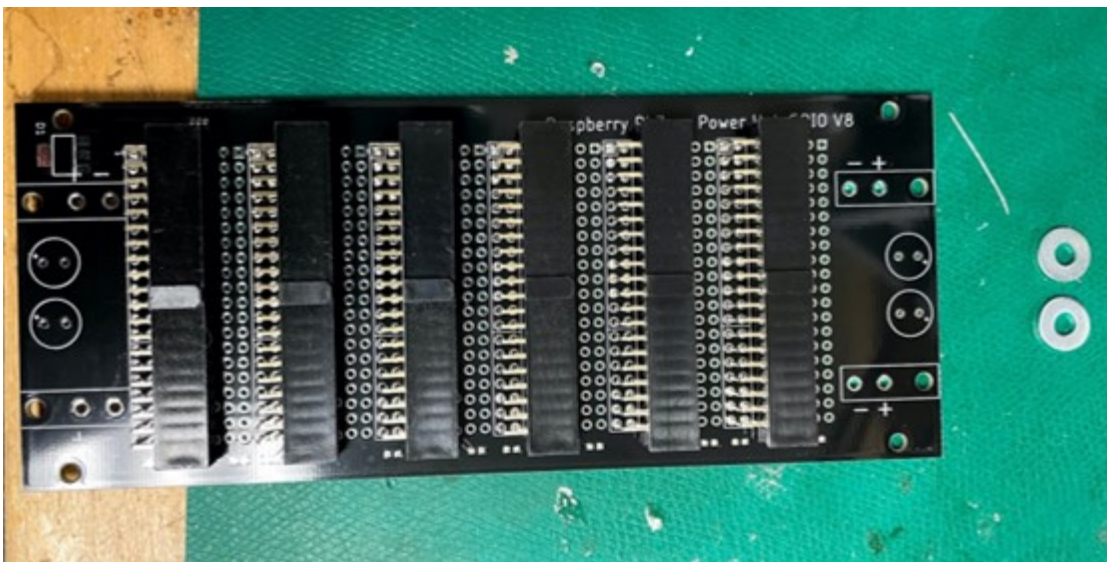
Figure A.11: Step#4: One side is complete
