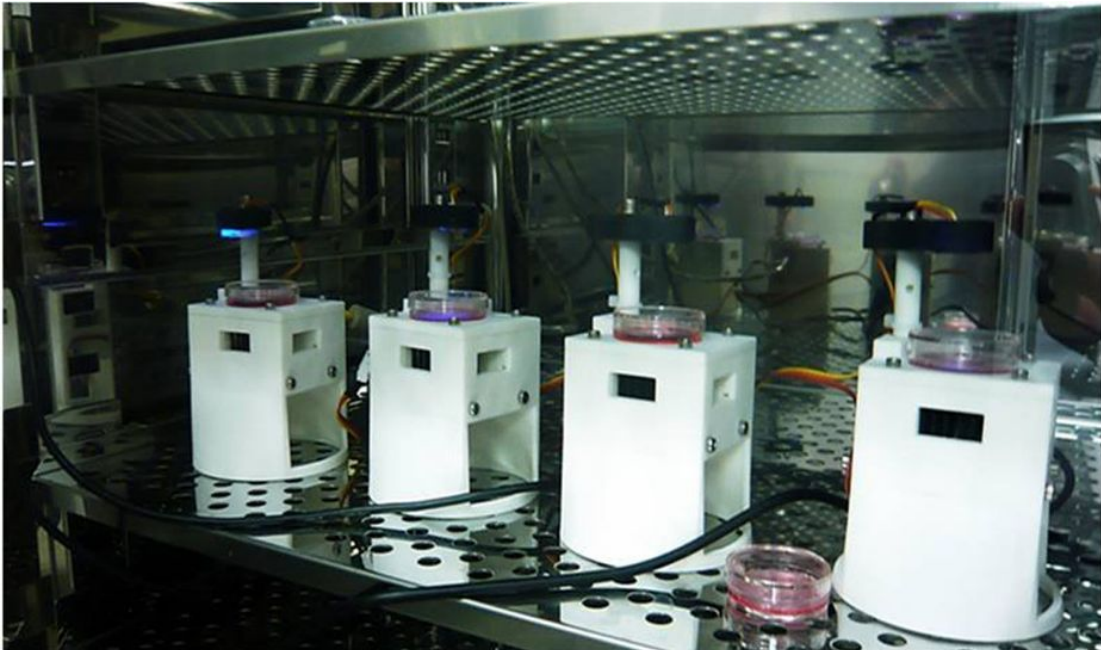
Figure 2.7: High-throughput lens-less microscope inside standard incubator [Kesavan et al., 2014]
