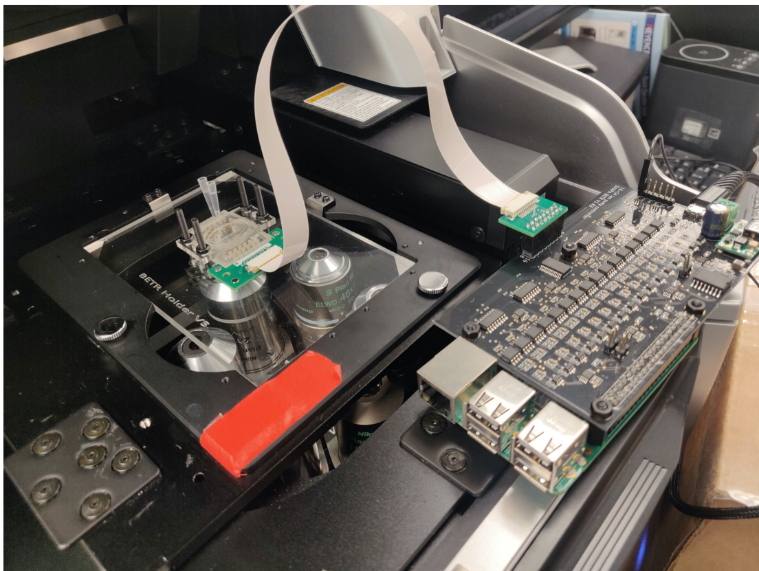
Figure 5.15: The non-modular multi-channel potentiostat connects to a vertical ion pump clamped on an acrylic holder mounted on the KEYENCE, BZ-X710 microscope.
