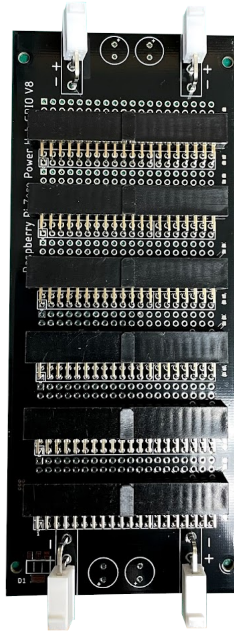
(b) Power distribution board
