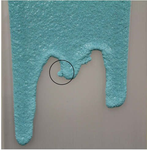
Fig. 4 Enlarged image of the ceramic beads showing clustering at \alpha = 50^\circ and \lambda = 0 ; the circled region shows the more prominent clustering features.
