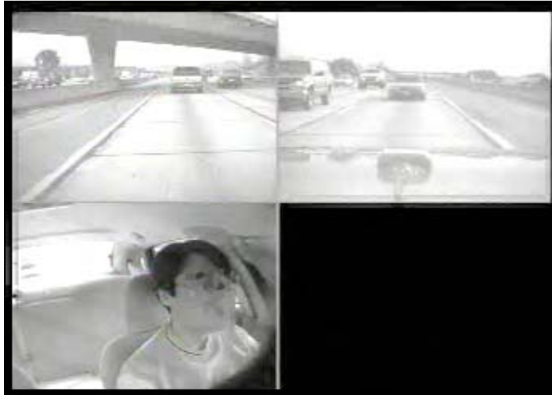
Figure 14. Captured frame from the 3 video cameras in the instrumented vehicle. Top left is front-view, top right is rear-view, and bottom left is the driver's face, distorted here to provide anonymity.
