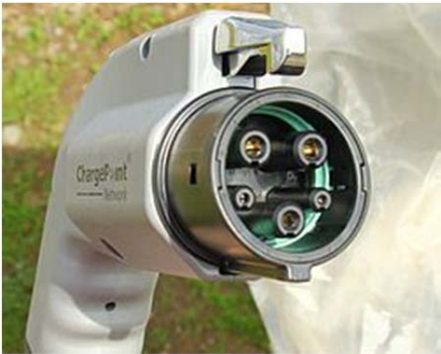
Figure 21. SAE J1772 PEV conductive charge coupler
