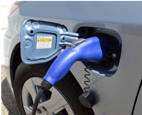
Figure 22. PEV charging coupler in use
