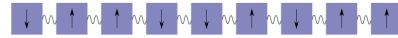
Figure 3.3: Transverse Field Ising Model. The blue squares represent a qubit with each line representing a state. The wavy line represents the interaction between qubits and the magnetic field is in the transverse direction.
