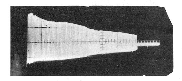
Fig. 3. Sweep trigger--end of rectification. Sweep speed 200 msec/cm. Sum induction-electrode signal of circulating proton beam tracked during the inversion period from 6.2 Bev down to 300 Mev.
