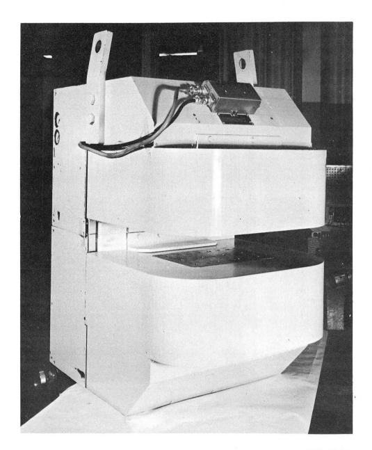
Fig. 2. New 9-by-12-inch bending magnet.
