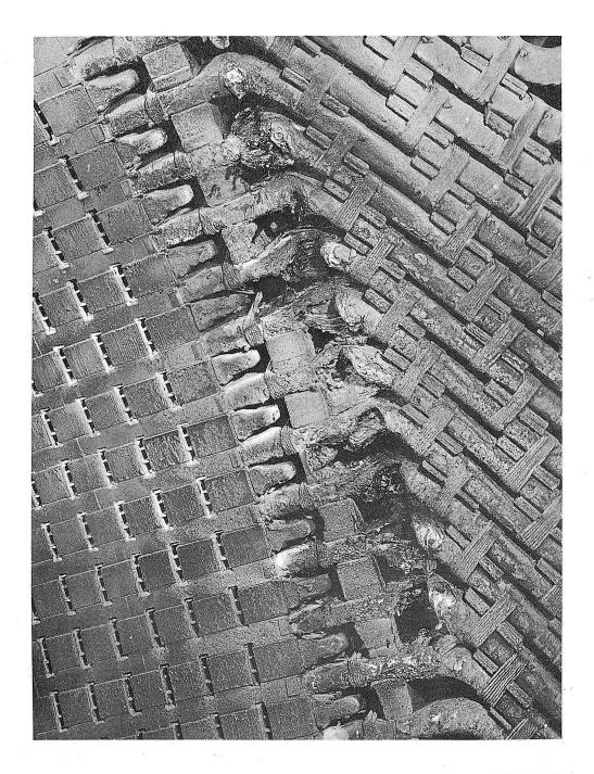
Fig. 4. Abrasion and fire damage to the stator of the west generator.
