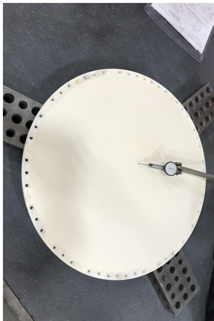
Figure 5.29: Curved surface indicator measurement on a granite table of a POLARBEAR-2b lens.
