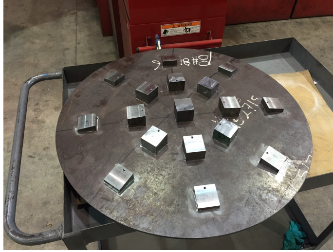
Figure 5.26: Curved fixture for large-scale thickness deposition uniformity testing on alumina coupons.
