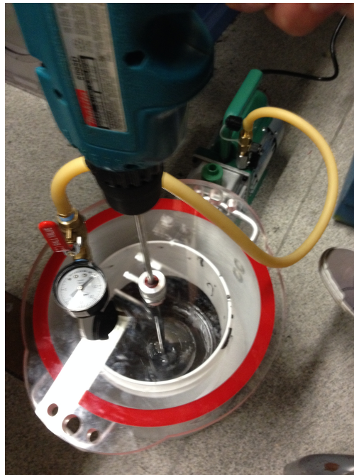
Figure 5.7: Epoxy mixing process inside vacuum chamber. The chamber has a vacuum-tight feedthrough for paddle rod attached to power drill, held by the author, which is utilized for a uniform mixing procedure.
