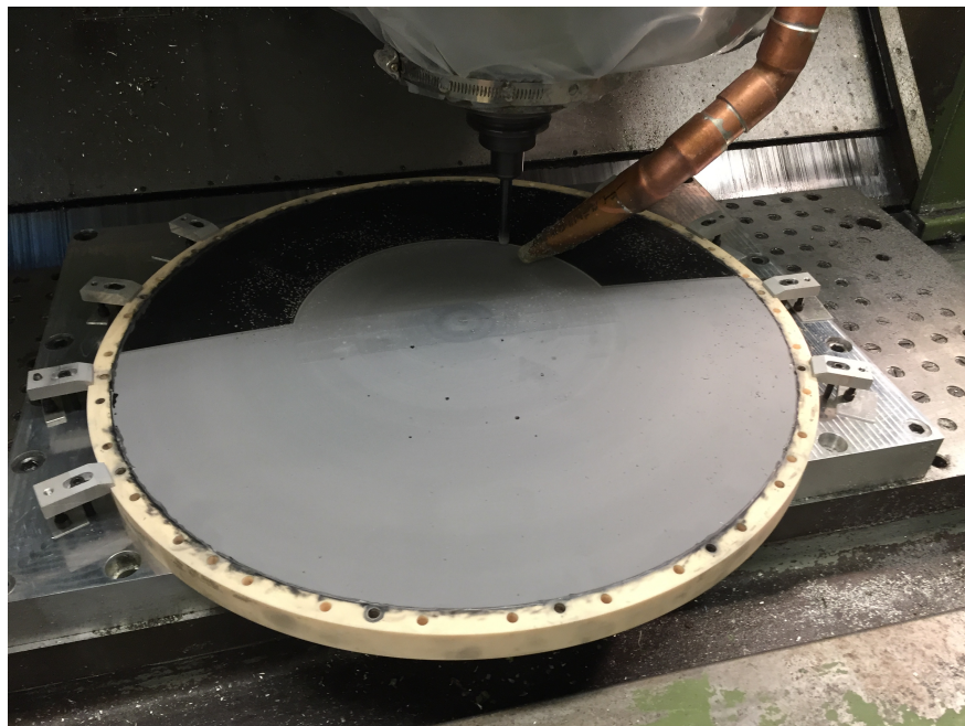
Figure 5.13: CNC machining in halves of the POLARBEAR-2a field lens.
