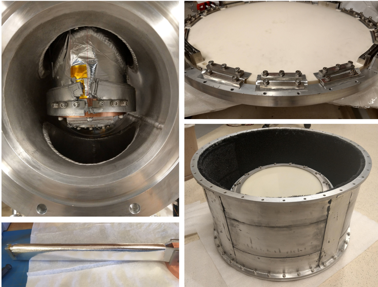
Figure 4.22: 6N Al use for lens thermal link, optics tube shells, heat links.
