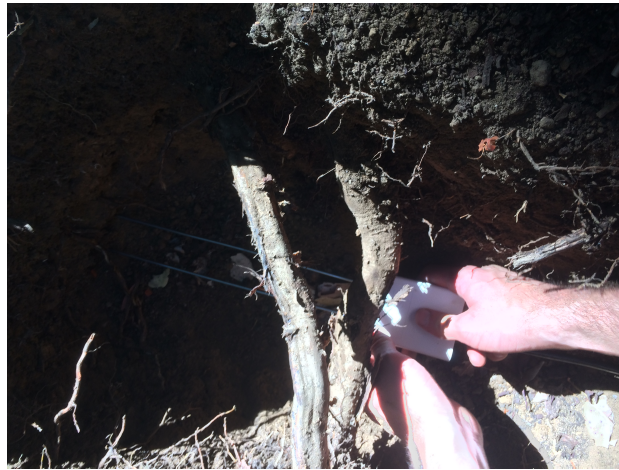
Figure 2.7: A shallow soil moisture probe pictured mid-installation, showing orientation of sensor before being inserted into the undisturbed soil of the pit wall. Large roots traversing the installation site were left intact.
