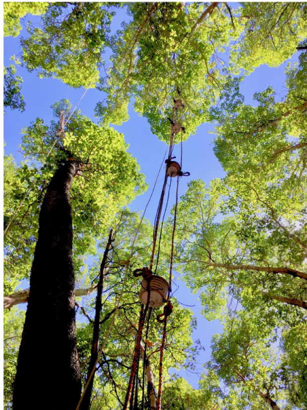
Figure 2.8: The top four in a string of 10 air temperature and humidity sensors, vertically suspended from a branch in the upper canopy, 25 m above the forest floor. Three strands keep the radiation shields in the correct upright position even under windy conditions.
