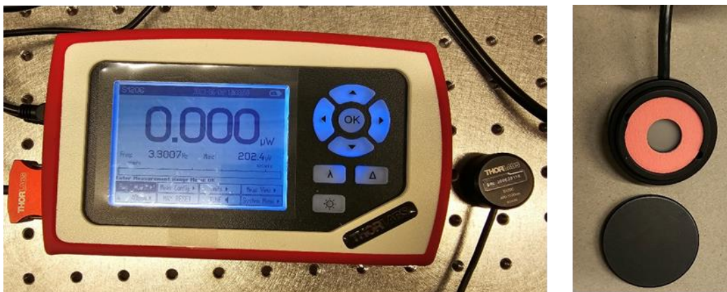
Figure 33: ThorLabs Photo detector and Power meter
