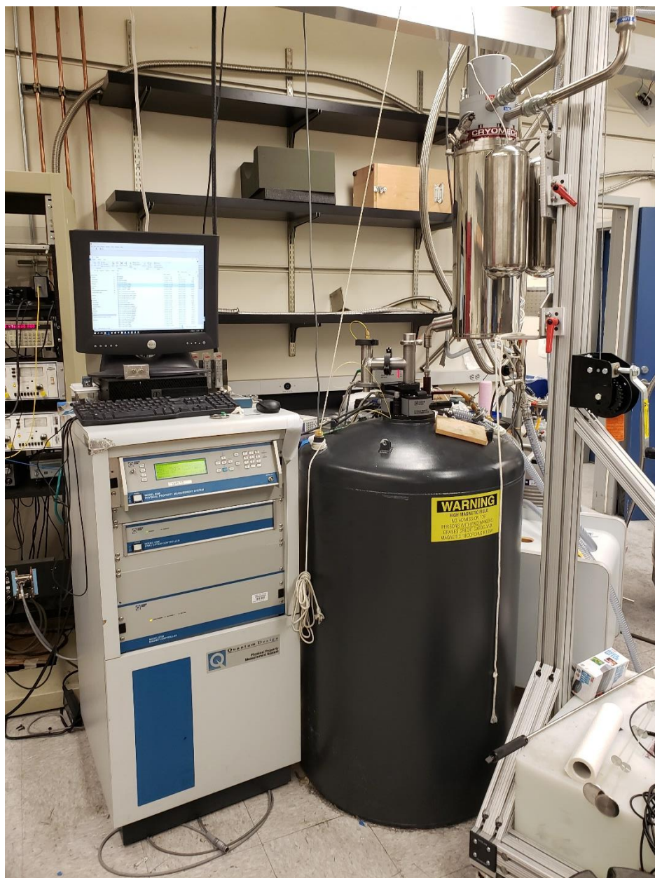
Figure 2.4: Picture of our Quantum Design PPMS fit with a CryoMech helium reliquifier allowing for extended time between liquid helium transfers.
