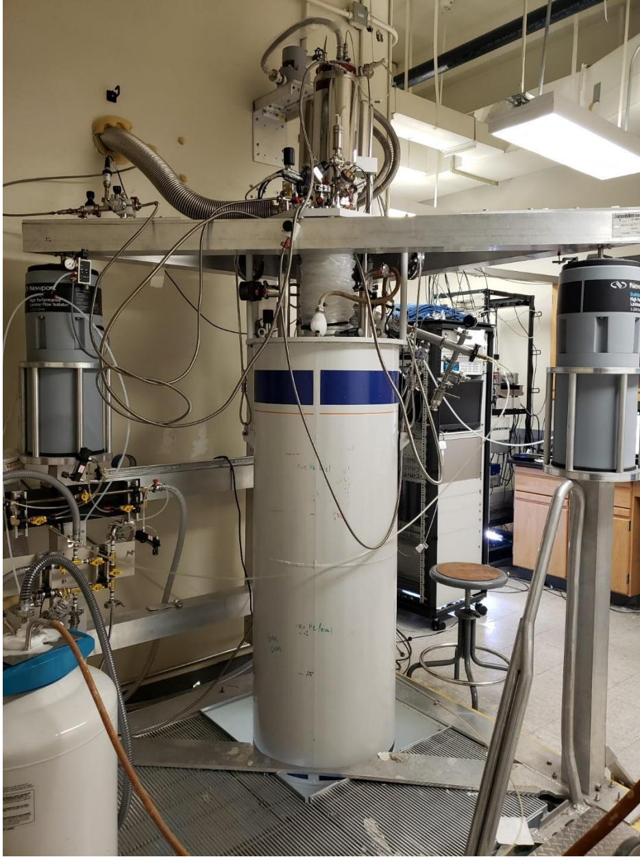
Figure 2.5 Oxford Dilution Refrigerator fit with a CryoMech helium reliquifier. The cryostat pictures here is set on a vibrationally isolated frame over a large pit which allows the helium dewar to be lowered, exposing the IVC and sample stage for use during sample changes.
