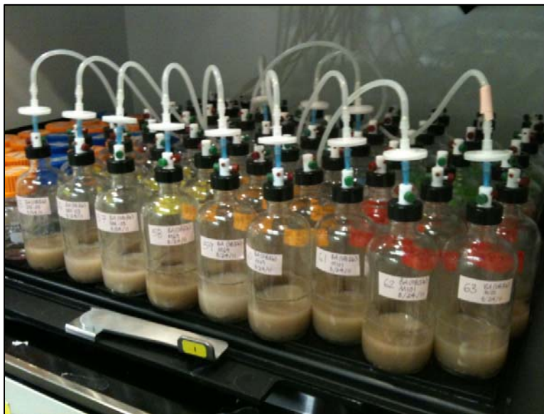
Figure 4.2. Microcosms constructed from AFP44 groundwater and soil on incubator shaker
