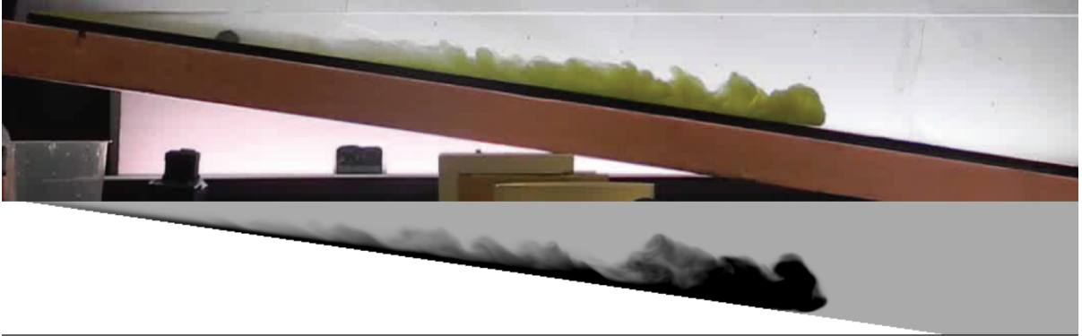
Figure 4.3: Snapshots of a turbidity current experiment (exp2, based on experiments by Snow and Sutherland [142], S = 0.176 , Re = 15,000 , v_s = 0.001 , m = 0.149 ) right before separation of the current from the bottom slope. Experimental results (top) and the corresponding numerical results are compared at time t = 12.1 .
