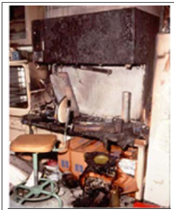
BSC fire. Source: Stanford University, Use of open flames in Cabinets/Tissue Culture Hoods (May 29, 2003).
