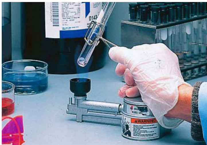
Touch-O-Matic Bunsen Burner. Source: Fisher Scientific (May 2010).
