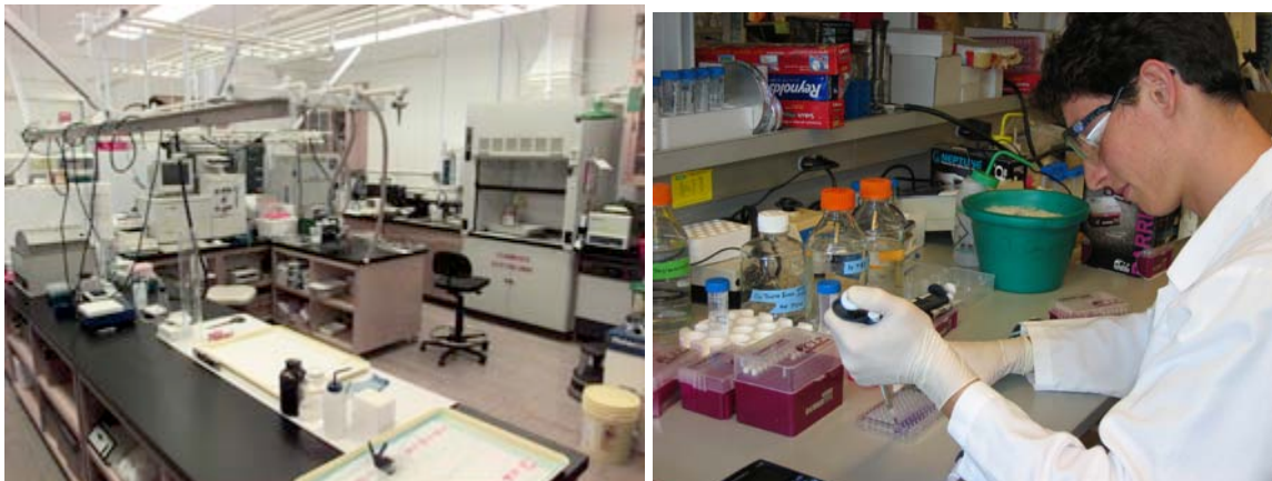
Laboratory Biosafety Level 1 work with open benchtops and standard microbiological practices. Source: LBNL EH&S.
