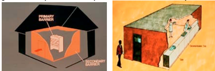
Standard facilities provide secondary barriers. Source: HHS CDC Office of Health and Safety.
