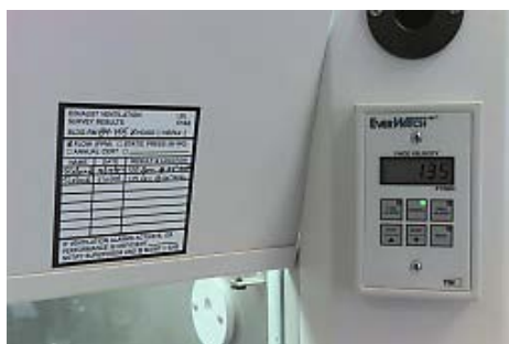
Hood survey label and monitor. Source: LBNL EH&S
