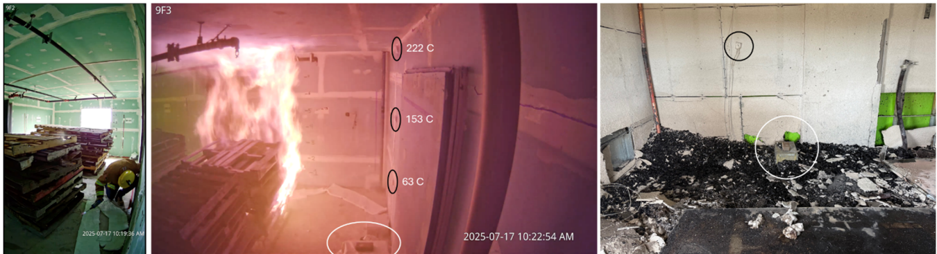
Figure 3. Still frames from cameras 9F2 (left) and 9F3(middle), and photo taken immediately post-test.
