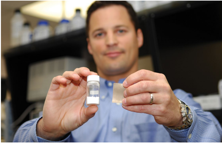
UCLA Professor Eric Hoek's low-energy, fouling-resistant nanotechnology membranes for desalination and wastewater treatment.
