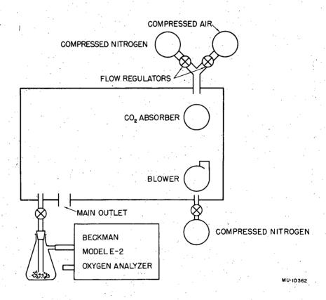
Fig. 6. Schematic diagram of the apparatus used to obtain an environment of low oxygen tension.
