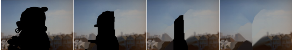
Figure 8.3: Filling \Omega_F for Image No.5 . From Left to Right: The intermediate result of inpainting at iteration 0, 20, 40 and final respectively. Left: \Omega_F . When inpainting starts, the algorithm fills the occluded region from outside to inside. Right: the inpainted \tilde{\mathbf{g}} .
