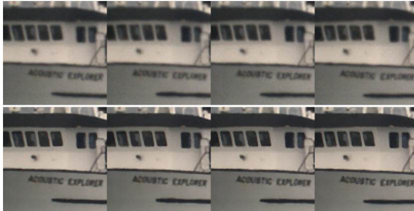
Figure 5.11: Zoom-in of “Acoustic Explorer” sequence frame no. 25-28 (object is 2 miles from camera). Top: input video sequence with contrast enhanced by gray level grouping (GLG). Bottom: Processed video by applying the proposed method to the output of GLG.
