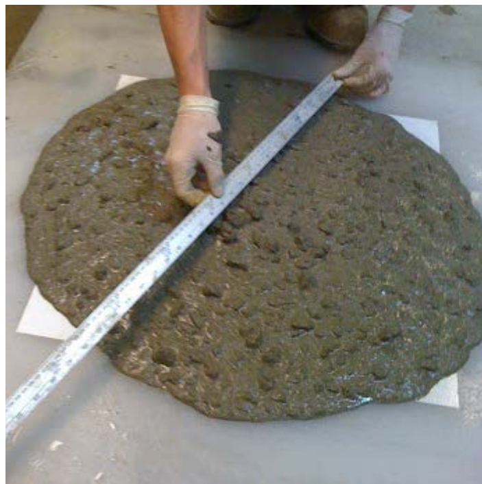
Figure 2.5 Slump flow test of self-consolidating concrete
