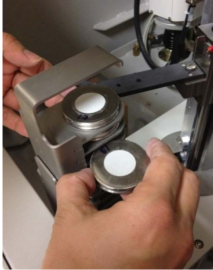
Figure 2.7 Placing finely-ground samples of cement paste mixtures into the diffractometer.
