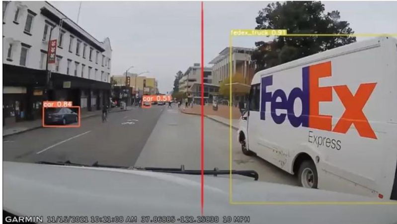
Figure 4. The bounding box includes the object’s label and confidence level
