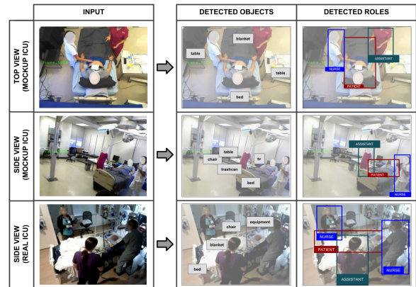
Figure 1: Views of the mock-up ICU room (top two rows) and the medical ICU room (bottom). The columns are the input frames (left), the detected objects (center), and the detected roles in the color bounding boxes (right).
