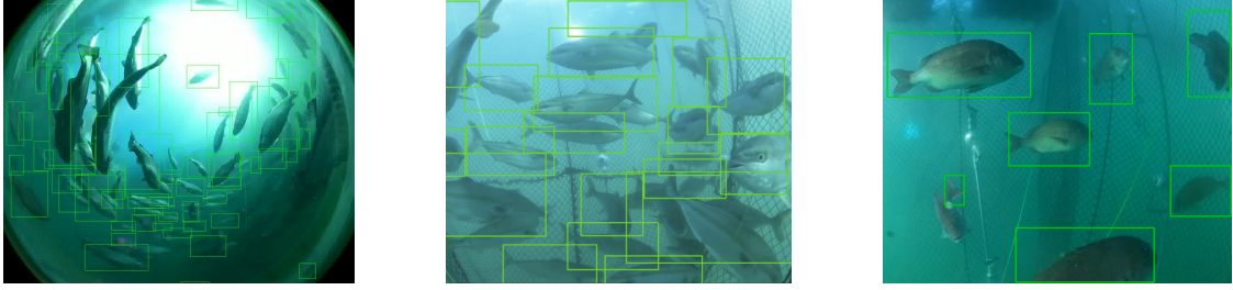
Figure 4.16: Example images of a fish counting system using the YOLOv4 trained model. The captured video data with (left) coho salmon (middle) yellowtail (right) red seabream were fed to our fish counting pipeline, and the total number of fish in each cage was estimated automatically.
