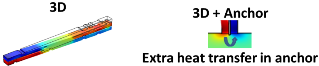
Figure 30: When the anchor is included in the simulation it allows for extra heat transfer lowering Q_{TED} and provides a more accurate simulation than when the anchor area is not included.
