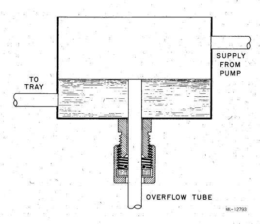
Fig. 4. Adjustable-level control for alcohol-tray supply.
